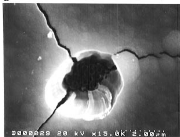
Figure 4. (a) Coating on contaminated surface viewed from top. (b) Same as in (a) with complete breakthrough of the coating down to support pore openings.
